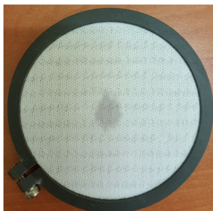
Figure 9. An example of wet spot on the fabric surface at 25% stretching after measurement using the MMT.
