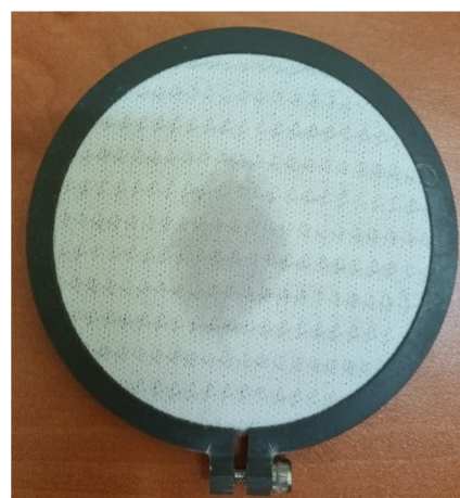
Figure 8. An example of wet spot on the fabric surface after measurement using the MMT.
