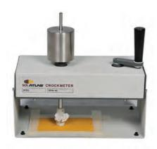
To determine the colorfastness of textiles to dry or wet rubbing particularly for printer fabrics. Applies 1134 grams of pressure on a 16 mm finger and rotate 1.125 turns clockwise then counter-clockwise. The operating handle is however turned in one direction only.
