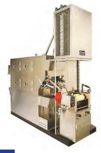
hermosol range with infrared zone suitable for working ut dye formulas and for research work.
