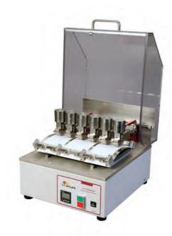
For evaluating a material's resistance to rubbing motion. Unit is a six station, benchtop machine which includes clamps for sample attachment to moving platen and clams for weighted rubbing arm for attachment of rubbing material. Cycle counter automatically stops machine at end of test cycles. Test samples are visually evaluated.
