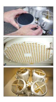
The Bundesmann provides a water repellency test for fabrics that are being contacted during use such as a rain jacket. Samples are mounted over a cup and are rubbed from underneath during the test. Three hundred precision stainless steel drop formers provide simulated rain falling from a height of 150 cm. Samples mount onto holders outside of the tester and then are easily set in place on top of the cups.
