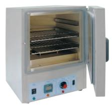
Dual purpose for both perspiration and oven-dry tests with high accuracy. 30 liter or 120 liter capacity. Dual temperature ranges and scales (25-110°C +/- 0.25°C, 50-250°C +/-0.75°C) stainless steel interior. Circulation fan and door thermometer, 2 shelves. Other sizes, temperature ranges and accuracies available upon request.
