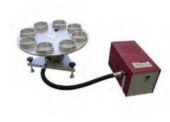
To determine the resistance of textiles and textile composites (particularly action wear fabrics) to water vapor penetration. The apparatus consists of 8 containers with water reservoirs, a standard permeable fabric cover, sample holder ring and precision drive system.
