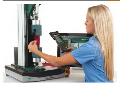
The ST series of electromechanical testing machines from Tinius Olsen are designed to test a wide range of materials in tensions, compression, flexure, shear, and peel.
