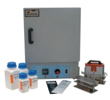
To determine colorfastness to water and perspiration of textiles. Provided with 2 stainless steel frames each with a capacity of 20 samples of 10 cm  $\times$  4 cm held between acrylic separator plates. Loading weights for BS, ISO and AATCC standards are included. An electric incubator is required available but not include.
