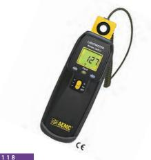
Lightweight and compact design, ideal for measurement of a wide range of lighting types with easy, one-hand operation. Removal sensor for remote reading with protection cover. Provides selectable lux or foot-candle units for display and features a 3 1/2 digit backlit LCD and HOLD function.
