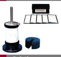
To determine a fabric's ability to recover after wrinkling under a predetermined load for a set period of time. Set of 3-D plastic replicas are available to grade fabrics.
