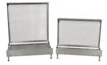
For determining the ignitability of material combinations for upholstered seating. The test rigs are covered with the standard foam and the fabric under test. The assembly is then ignited using one of the standard ignition sources and the combustion process is monitored.
