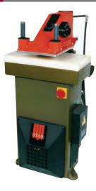
Swing arm cutting presses are ideally suited to cutting test samples from textiles. Rubbers and soft plastic prior to testing. Depending on resilience, several thicknesses can be cut at once with a cutting force of 20 tons. Control push buttons with time delay ensure complete operator safety. Maximum cutting area 18" (450mm) x 36" (900mm). Cutting dies of any shape and size can be supplied.
