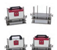
To determine the colorfastness to water and perspiration in textiles. A stainless steel frame with a capacity of 20 samples of 10 cm  $\times$  4 cm held between acrylic separator plates, loading weights not included. Comply with AATCC and ISO test methods by add on individual weights: 3.36 kg (8 lb) for AATCC, and additional weight 0.47 kg (1 lb) for ISO. An electric incubator is required.
