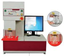
The Autoburst is a hydraulic bursting tester with advanced testing controls. The instrument has automatic flow control allowing bursts to be achieved within the specified time of the standard. The advanced software provides diaphragm correction calculations for consistent results. These features, along with a maximum capacity of 6000 kPa (871 psi), make the Autoburst the most versatile burst tester on the market.
