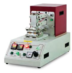
The UWT is used to test wear and abrasion resistance of fabrics for apparel, shoes, upholstery, automotive, and many other areas. The instrument, also known as a Stoll Quartermaster Abrasion Tester is designed to run numerous tests with five different possible setups.
