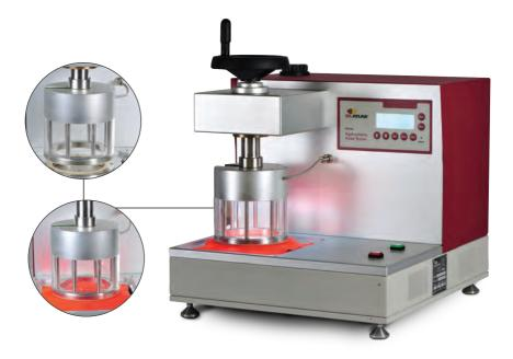
Powerful and intelligent, the Hydrostatic Head Tester is designed to help labs be more efficient while meeting global standards. The compact design can reach 3 bar of pressure using standard lab compressed air. The quicktest function allows users to perform other tasks during the first 80% of the standard test. An alarm indicates fail pressure is close and a technician should begin observing. The test area is well lit behind a clear shield for observing when droplets appear.
