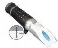
To determine the amount of starch or solids percentage in a sizing solution.
