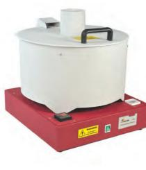
STANDARDS: BS 1006 UK/TN CPS+ Benchtop Xenon Arc system is the ideal instrument for initial accelerated lightfastness and photostability testing. It features:
