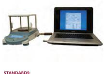
Consists of an electronic balance (220 grams x 0.001 grams) with internal and external custom software which calculates yarn, sliver and roving counts as well as fabric yield in various systems and provides statistics on any number of tests including totals, average, CV and SD. Includes cables and security data key, USB, and connects to any PC and printer. PC and Printer are not available.
