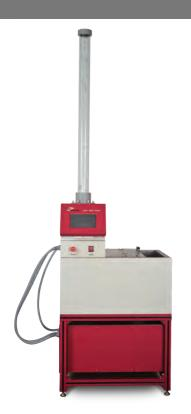
The Rain Tester provides a water repellency test for fabrics with different intensities of water impact at specified water temperature. Samples are mounted vertically while the simulated rain is sprayed horizontally. Samples are backed with a standard blotting paper that is weighed before and after the test. The Rain Tester provides precise control of the test through a color touch screen controller including water column height, water temperature, and test time.
