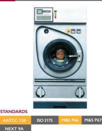
For conditioning textiles to consistent temperature and humidity for accurate color measurements. Allows user to set specifications based on temperature and humidity and achieve these conditions in minutes. Standard temperature and humidity settings 20 deg. C, 70 deg. F, 65% RH, variable settings as per chart require option M222RCV. Fabric sample size range up to 9" x 12" to 20 specimens per cycle depending on sample weight and size.
