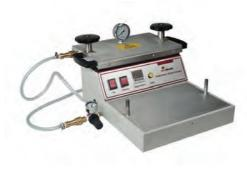
To distinguish between imperfections in fabric construction and streaking due to dyeing and finishing. By the controlled application of heat, pressure and cooling, a permanent impression of a test fabric is made from Optical quality polystyrene film, allowing objective analysis of external imperfections without the confusion of color or pattern.
