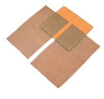
When a sample is observed to have lost color or have changed color during washing, this may be due to the effect of washing or the effect of the presence of optical brightener on the sample. This can be assessed using the fluorescence suppressor.
