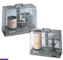
To determine and chart temperature and relative humidity over a selected period. Dual chart switchable, 1 day or 7 days with quartz clock, drive charts and pens  $0-40^{\circ}$ C,  $0-90^{\circ}$  RH.
