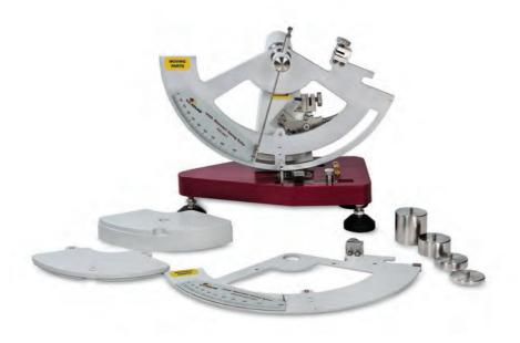
To determine the ballistic tearing strength of textiles, paper or board. Three interchangeable pendulums ranging from 8,000 to 64,000 Millinewtons (mN) can be selected seperately for multiple test method compliance.
