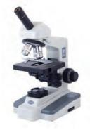
For the examination of textiles up to 1000 times magnification. Eye pieces 10x, objectives 4x, 10x, 40x and 100x, 12V/20W Halogen illumination with intensity adjustment,  $45^{\circ}$  inclined Monocular head with  $360^{\circ}$  rotatable head, coarse and fine focusing, vertical travel range 27mm.
