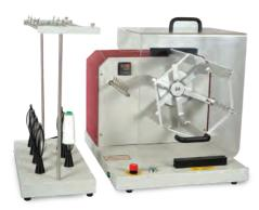
To produce skeins of yarn of a predetermined length and number of turns for count and/or strength testing. 1 Meter, 36" or 54" circumference collapsible swift (specify). Complete with yarn package stand and pretension device, fitted with predetermined counter. Available win hand operated and electronic versions.
