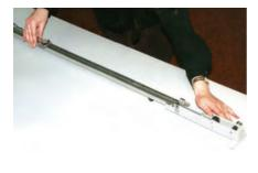
To calculate the crimp in yarn affected by knitting or weaving, to determine actual yarn usage. Threads are removed from a strip of fabrics of known length, straightened by a tension, then measured in the straightened state. Two tension ranges available (0-35 g and 0-175 g) and test length is 120 cm (48 inches).
