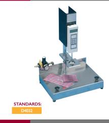
Determines fabric stiffness using the ASTM circular bend test method. A plunger of 25.4mm (1 in) diameter pushes the fabric through a 38mm (1.5 in) diameter orifice for a distance of 57mm (2.25 in) in 1.7 seconds, and the maximum force is recorded. Provided with pneumatic cylinder, controls and battery-operated digital force guage (switchable) 50 kgf / 500 N / 100 lb or 25 kgf / 250 N / 50 lb with peak-hold facility.
