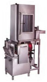
Heavy duty padder with stand, for all dyeing, impregnating and padding processes. Floor model.
