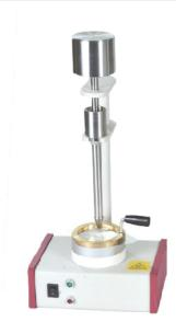
To determine the oil or finish content of wool or synthetic samples by solvent percolation and evaporation. Suitable for fiber, yarn or fabric. Available with 1, 2 or 3 extraction units. To be fully compliant with Edana method ERT 155, it needs a large extraction tube- 12 mm (OD), 10 mm (ID). (Full title of new method is: DETERMINATION OF ACETONE EXTRACTABLE FINISH ON NONWOVENS).
