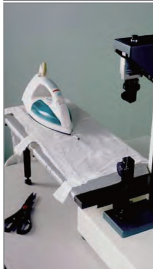
Iron friction test
