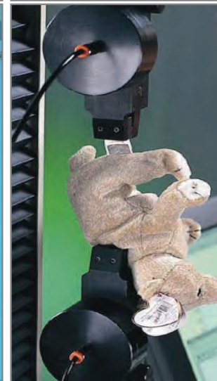
Toy Tests using pneumatic grips
