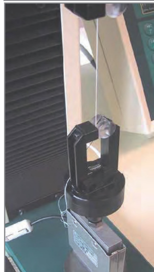
Elastomer Fibre tests using pneumatic grips
