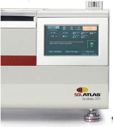
The DryRate 201 testing conditions are constantly monitored by the built-in anemometer (air flow sensor) and infrared thermocouple probe.
